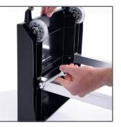
Connect the two aluminum guad tubes into the corresponding openings of the two stand modules. Fix the self-tapping screws (4.2 x 16 mm) with a 7 mm jaw wrench and a washer on the outside.
