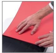
Now remove the supporting film from the EVA mat and glue them to the center of the wheel. There are about 3-4 mm of space on each side of the EVA mat. If necessary trim the last part of the EVA mat before pasting it.
