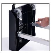
Then fix the self-tapping screws (4.2 x 16 mm) with a 7 mm jaw wrench and a washer on the inside.
